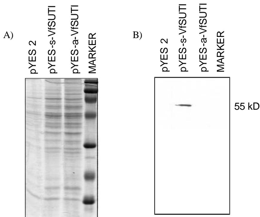
*Fig. 3.2.1.4 Cross-reactivity of the peptide antiserum SUT-XI with the VfSUT1 protein produced in transgenic yeast cells. (A) Coomassie stained gel showing the pattern of the total protein isolated from yeast cells. (B) Western blot analysis of VfSUT1 protein expression in yeast cells transformed by pYES-A-VfSUT1 or pYES-S-VfSUT1 using SUT-XI as primary antibody.*
