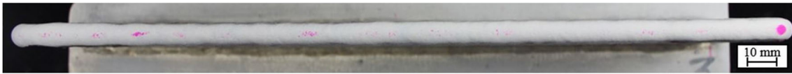
Fig. 8 Result of penetration testing of the last layer surface (S Ni 6625 AM2 with wire feed speed: 7.5 m/min, travel speed: 13 mm/min, heat input: 0.18 kJ/mm)
