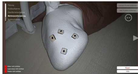
(c) Partially occluded phantom with simulated adhesive markers. The image also shows the GUI that is displayed while the user records the marker positions.
