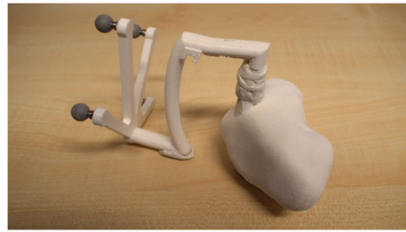
(a) Kidney phantom with the adapter for externally visible tracking markers
