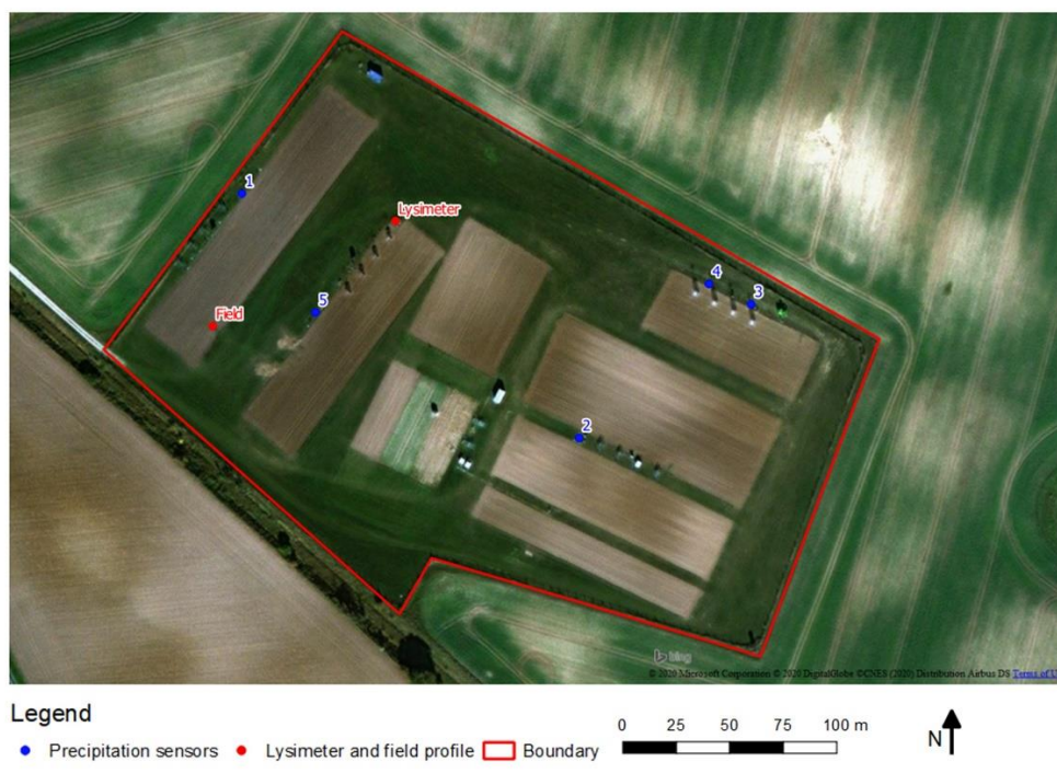
Figure 3.2: Aerial image (capture date range: 30 June 2010 to 19 Sept. 2016) and map of the experimental field site (CarboZalf-D) located in northeastern Germany; the locations of the rain gauges and the “field” soil profile and “lysimeter” station. Locations of rain gauges for measuring precipitation are numbered (1–5), and instrument types are described (Appendix A3.2).
