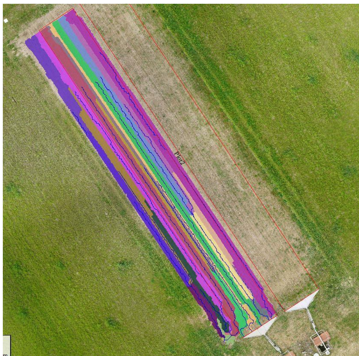
A2.1: Potential flow lines at the soil surface of the hillslope runoff experiment determined from a digital elevation model (GlobalMapper 19.0, LiDAR, 2018, resolution: 1.2 cm x 1.2 cm).
