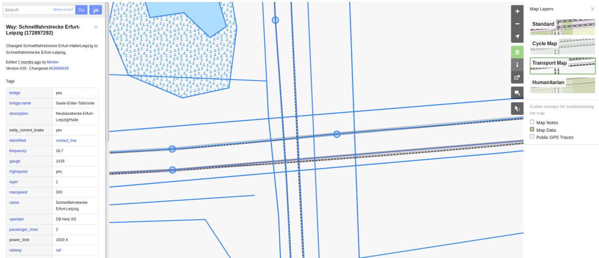
Fig. 3.1: Screenshot(©OpenStreetMap contributors) from the OSM in map data mode. We can identify single tracks and find useful metadata. This data states that the tracks cross via a bridge with an ICE track of the DB Netz AG with a max speed of 300 km/h. Image [Ope19]
