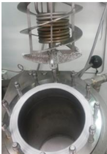
Figure 11. 5-liter Büchi reactor, power compensation heating element, double ribbon helical stirrer
