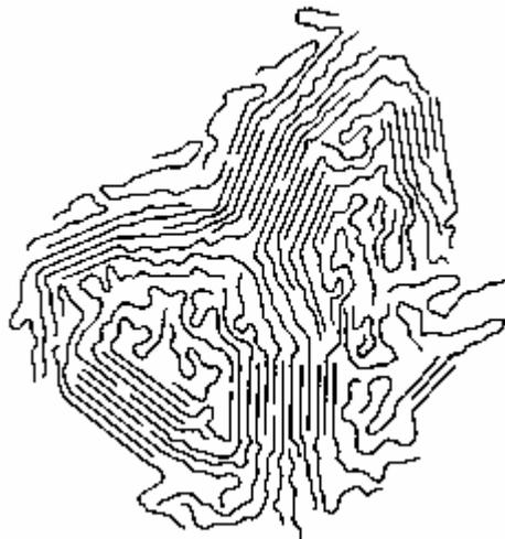
**Figure 1.1** A semi-crystalline polymer containing amorphous and crystalline regions
