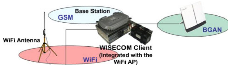
Figure 5. System architecture for the BGAN configuration.
