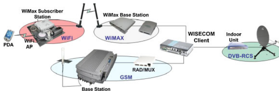
Figure 6. System architecture for the DVB-RCS configuration.
