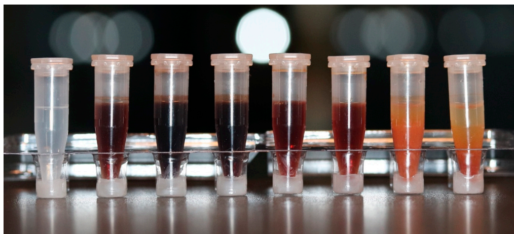
Figure 3. Microtubes containing 2% CHX mixed with different concentrations of NaOCl, to illustrate the precipitate formation. From left to right: (1) control sample with 0% NaOCl; (2) 0.5%; (3) 1%; (4) 1.5%; (5) 2.5%; (6) 3%; (7) 4%; (8) 5%.
