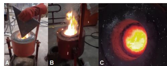
Figure 1: Obtaining of the Termites: A) Reactor feed and ignition of the reaction, B) Self sustainability of the reaction, C) Cooling of the termite
