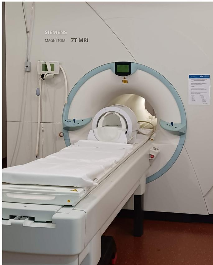
**Figure 2.1:** Utilized 7 T Siemens MAGNETOM MR scanner with NOVA Medical head coil.
