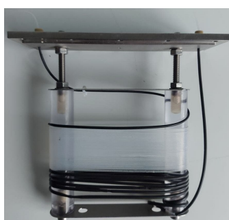
(a) Frame integrated in the photoreactor
