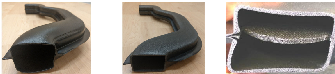
Figure 10: Solid HDPE duct (left), ALVEOLEN foam duct (middle) and ALVEOLEN foam duct with interlayer insert (right)
