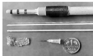
Fig. 2 Sensor with three electrodes for drop tower experiments
