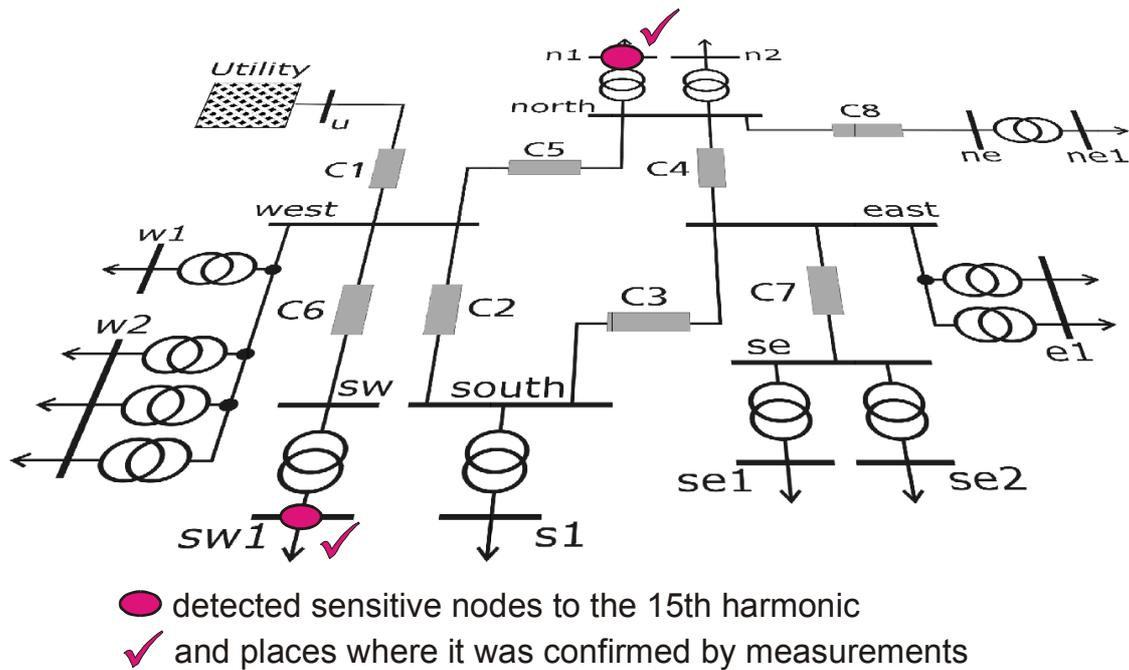
Fig. 5.18 Comparison measurements – sensitivity analysis, 15<sup>th</sup> harmonic case
