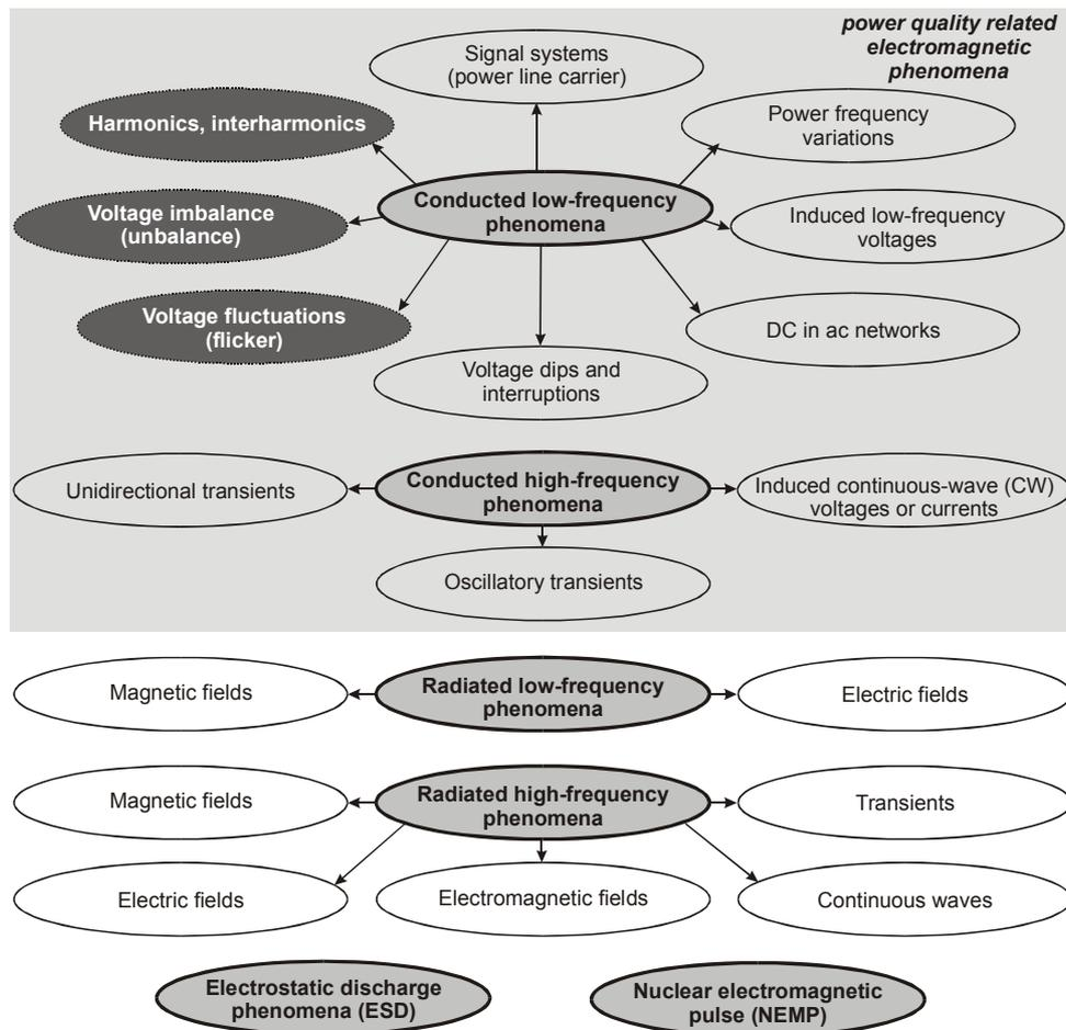
**Fig. 2.1 Principal phenomena causing electromagnetic disturbances as classified by the IEC [23] and fields of interest of this work**
