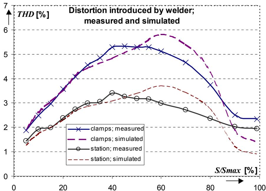
Fig. 4.8 Comparison between measurements and simulation results: Voltage distortion at both ends of the supply cable (points A, a in Fig. 4.6)
