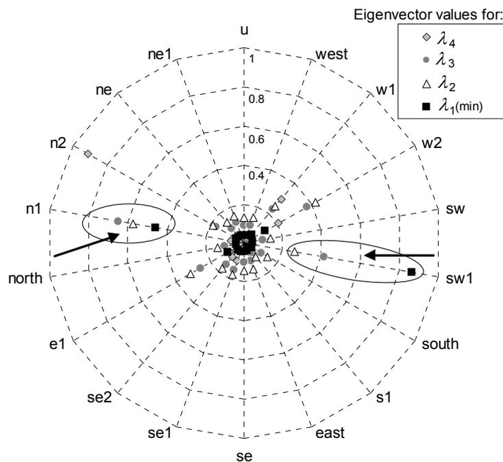
**Fig. 5.20 Eigenvector values that correspond to the four smallest eigenvalues, analysis for 15<sup>th</sup> harmonics**
