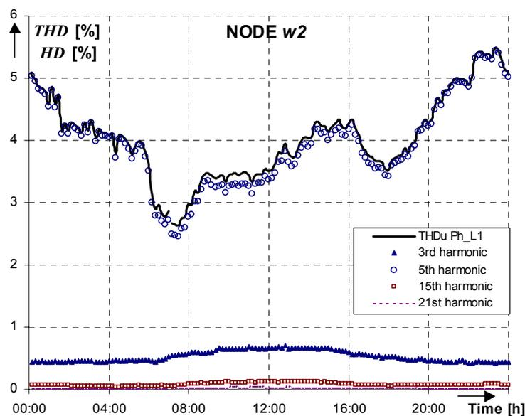
Fig. 5.9 *THD* and *HD* factors at node *w2*
