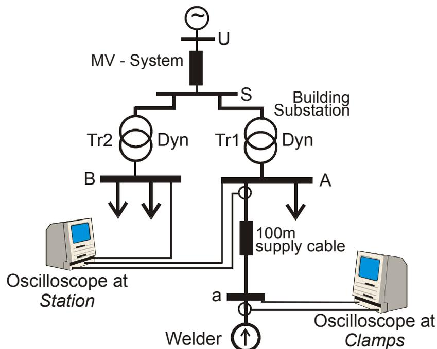
Fig. 4.6 Measurement setup in the studied distribution system
