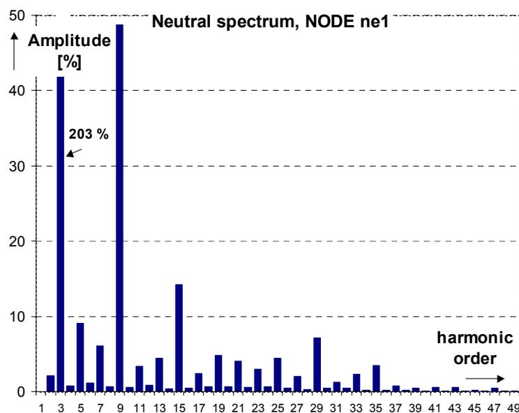
Fig. 5.13 Spectrum of the current flowing in neutral conductor at node *ne1*
