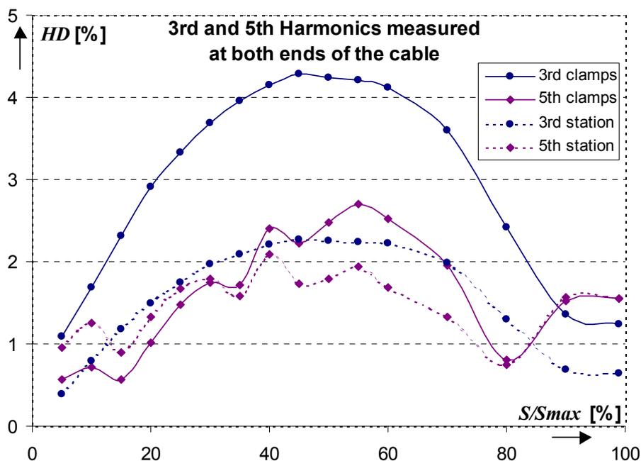
Fig. 4.7 Harmonic content of the voltage measured at the clamps (a) and station (A)
