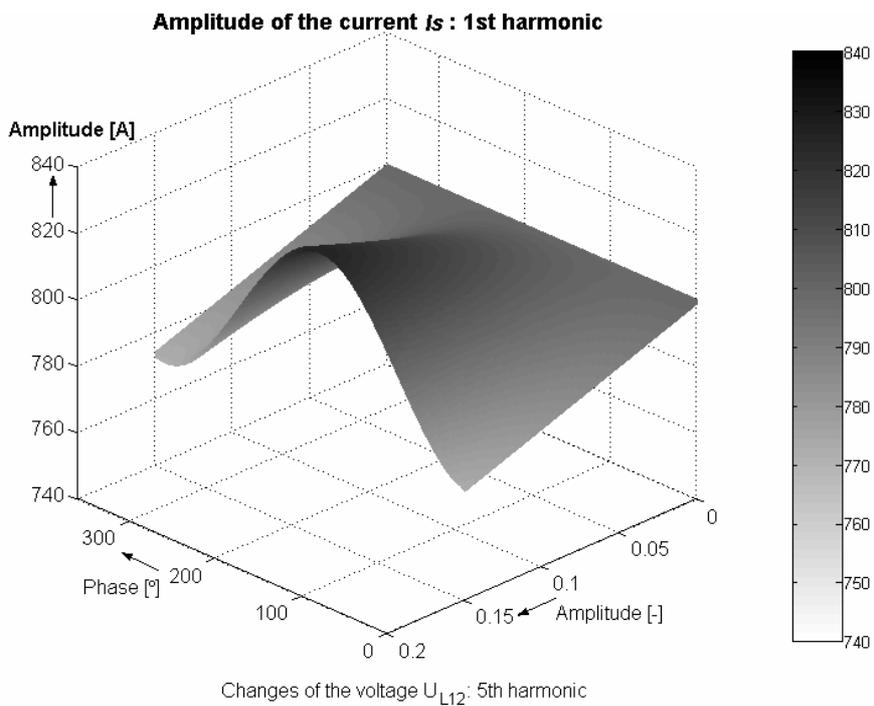
**Fig. 4.18 Influence of the 5<sup>th</sup> harmonic voltage  $U_{L12}$  changes on the first harmonic current drawn by the machine**
