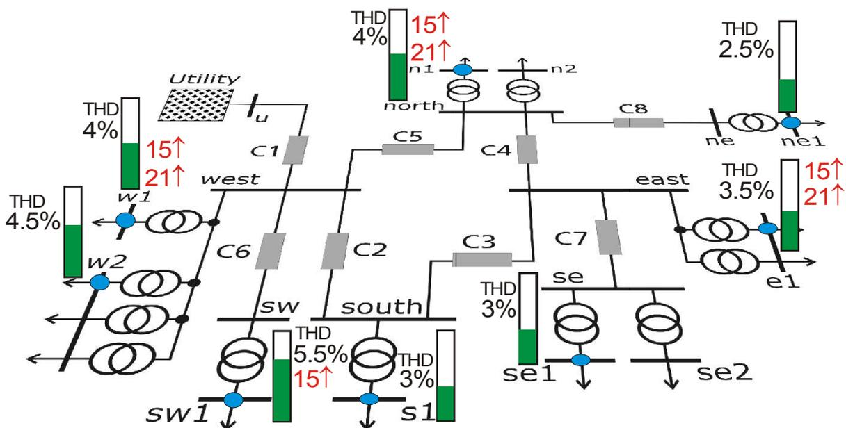
Fig. 5.5  $THD$  level within the distribution network
