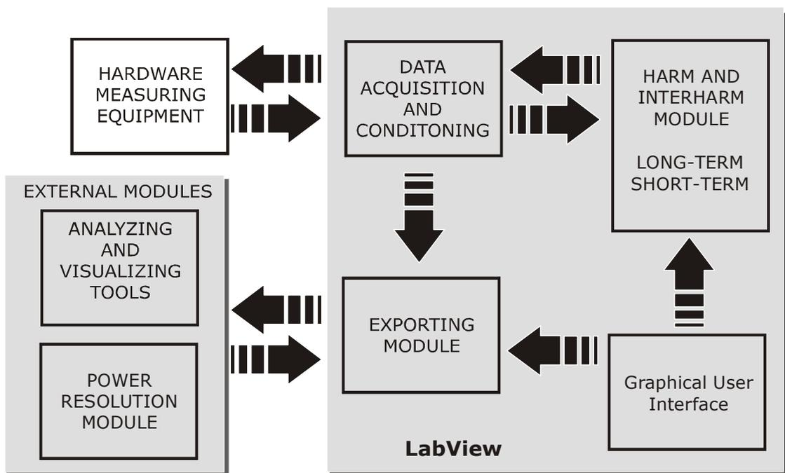
Fig. 3.1 Power quality monitoring system - general scheme
