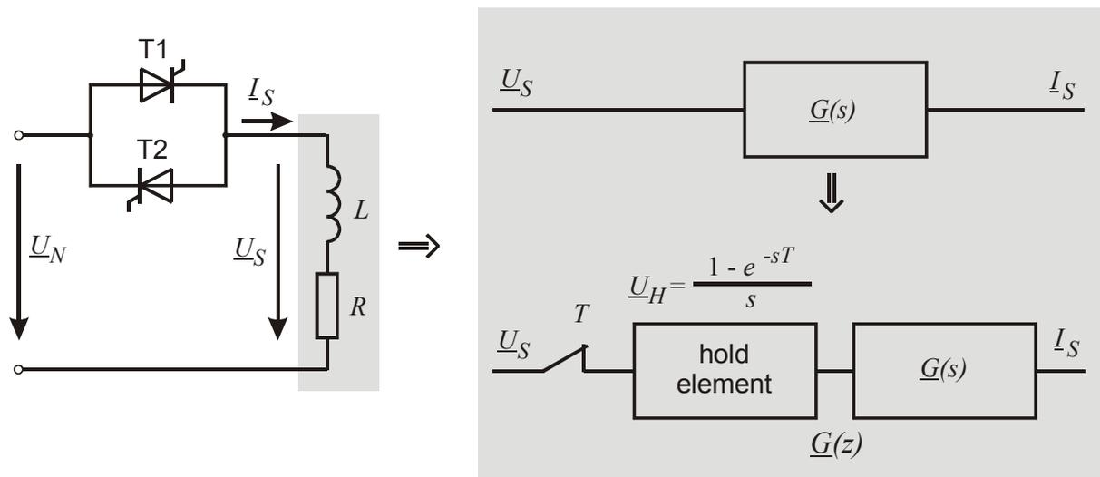
**Fig. 4.13** Parameterization of the welding machine and transmittance based procedure for the measurement-based parameter identification
