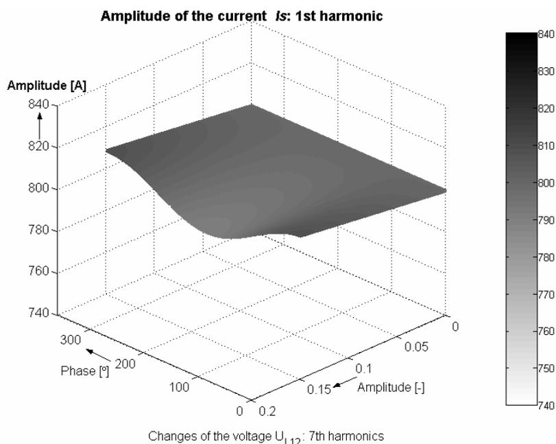
**Fig. 4.20** Influence of the 7<sup>th</sup> harmonic voltage  $U_{L12}$  changes on the first harmonic current drawn by the machine
