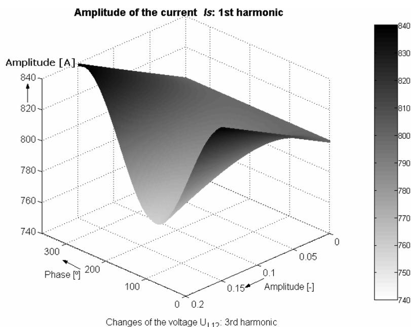
**Fig. 4.19** Influence of the 3<sup>rd</sup> harmonic voltage  $U_{L12}$  changes on the first harmonic current drawn by the machine
