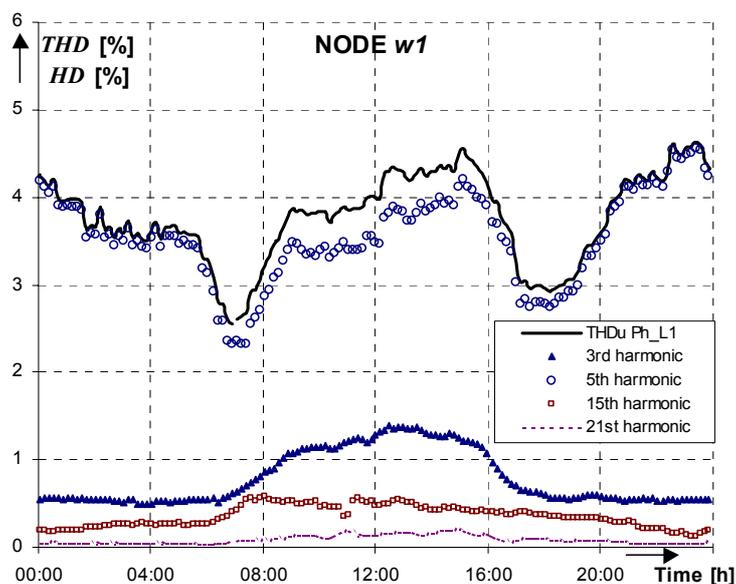
Fig. 5.6 *THD* and *HD* factors at node *w1* for phase L1
