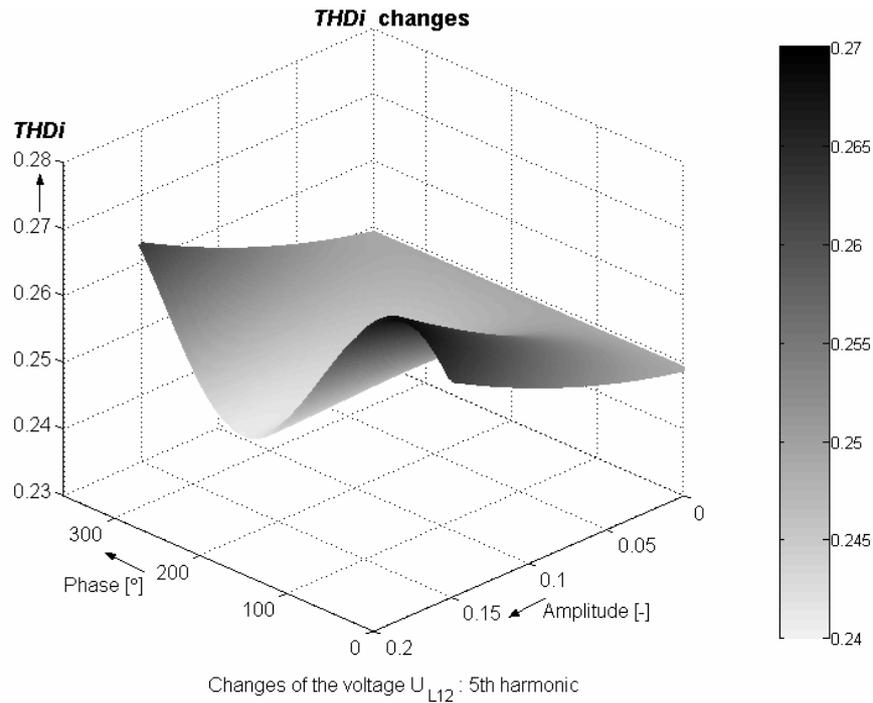
**Fig. 4.17 Influence of the 5<sup>th</sup> harmonic voltage  $U_{L12}$  changes on the  $THDi$  of the current drawn by the machine**
