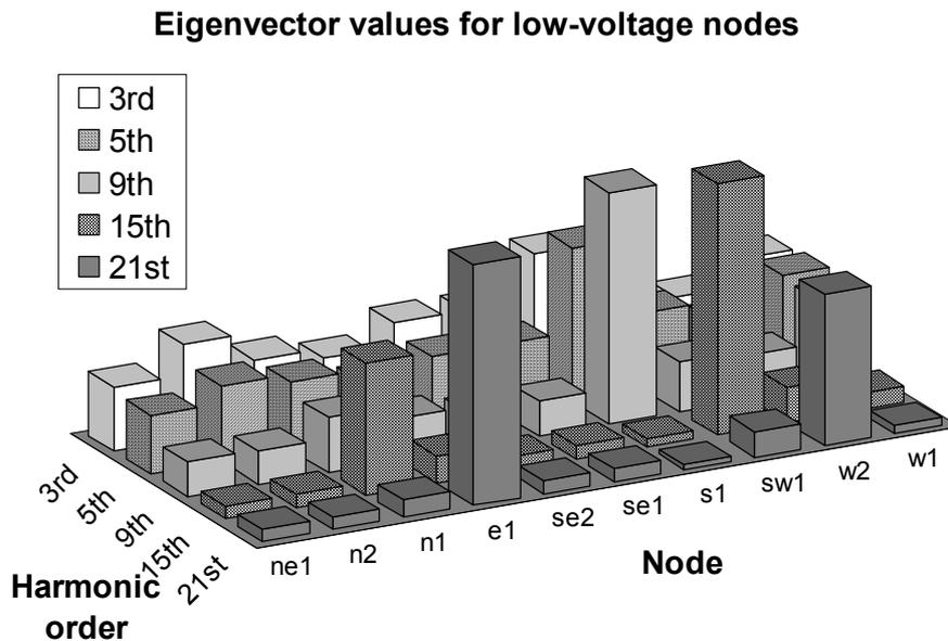
**Fig. 5.16** Eigenvector values for the minimum eigenvalue calculated for low-voltage nodes in the studied system at chosen harmonic orders
