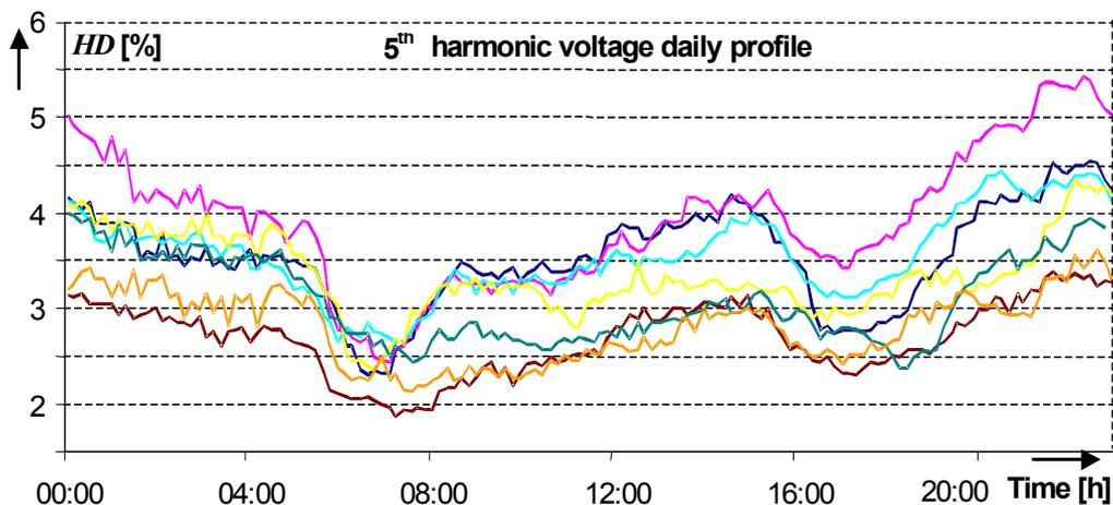
Fig. 5.15 Level of the 5<sup>th</sup> harmonic at every site
