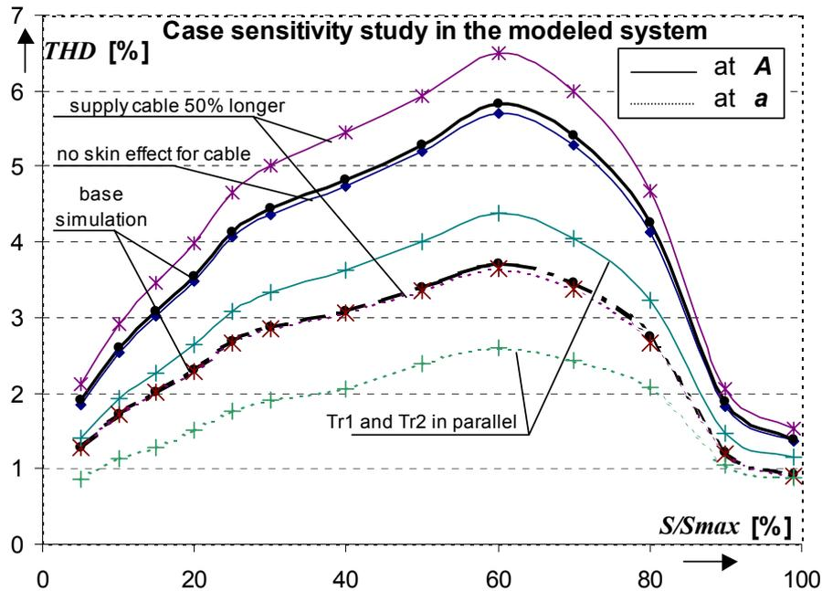
Fig. 4.9 Influence of the model parameter on the harmonic distortion at the clamps (a) and at the bus (A)
