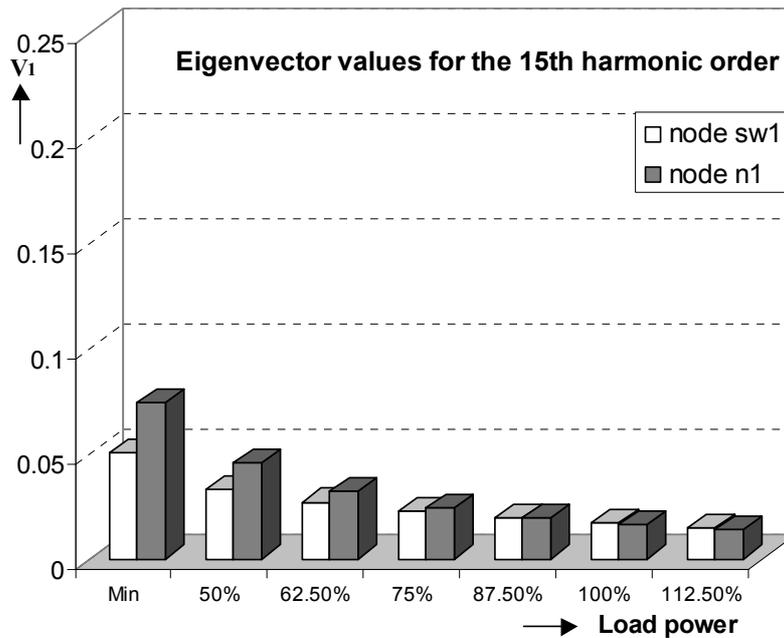
Fig. 5.24 Eigenvector values changes as a function of the non-linear load power calculated for 15<sup>th</sup> harmonic order
