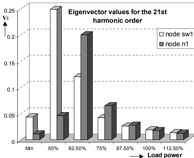
Fig. 5.25 Eigenvector values changes as a function of the non-linear load power calculated for 21<sup>st</sup> harmonic order
