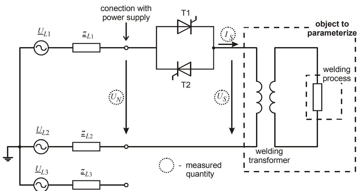
Fig. 4.12 Measuring arrangement for the identification of the welding process' parameters
