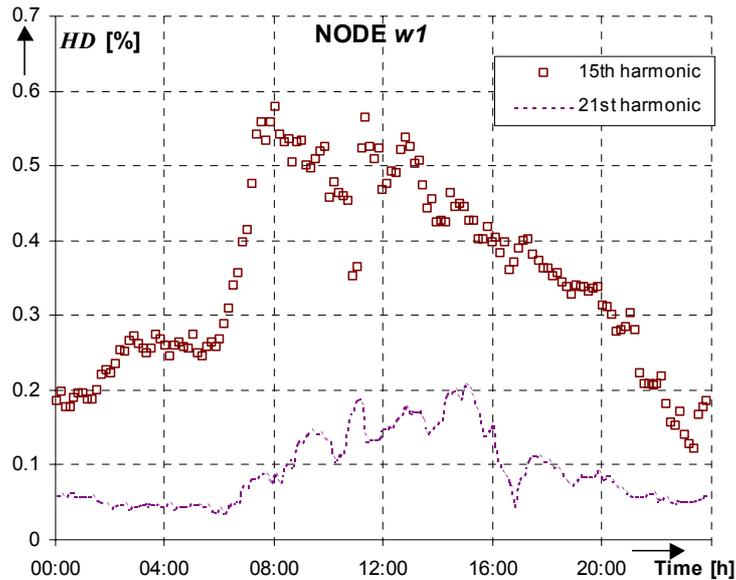
Fig. 5.7 *HD* factors for 15<sup>th</sup> and 21<sup>st</sup> harmonic orders at node *w1*
