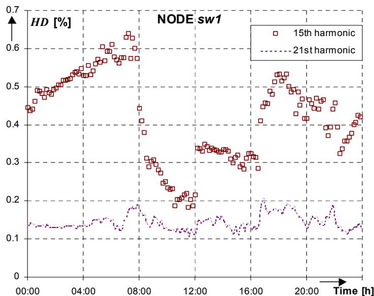
Fig. 5.11 *HD* factors for 15<sup>th</sup> and 21<sup>st</sup> harmonics at node *sw1*
