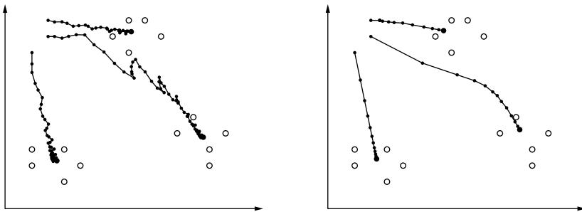
Figure 5.9: Learning vector quantization with 3 reference vectors for a simple set of 15 data points. Left: online training with (constant) learning rate  $\eta_{\vec{\mu}} = 0.1$ , right: batch training with (constant) learning rate  $\eta_{\vec{\mu}} = 0.05$ .
