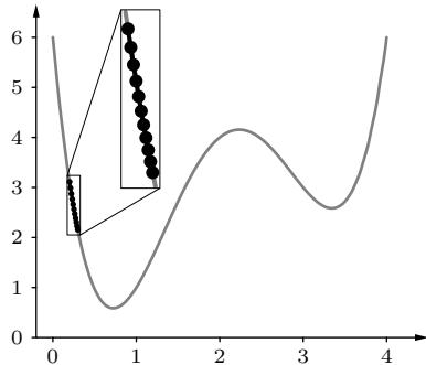
Figure 5.2: Gradient descent with initial value 0.2 and learning rate 0.001.
