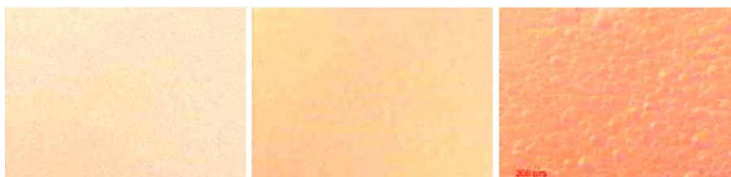
Fig. 6.12. The colors of the ZnO films grown with increasing amount of ammonia (from left to the right). Growth temperature: 850 °C. Ammonia flows: a): 0.9 mmol/min, b): 1.6 mmol/min, c): 3.2 mmol/min.
