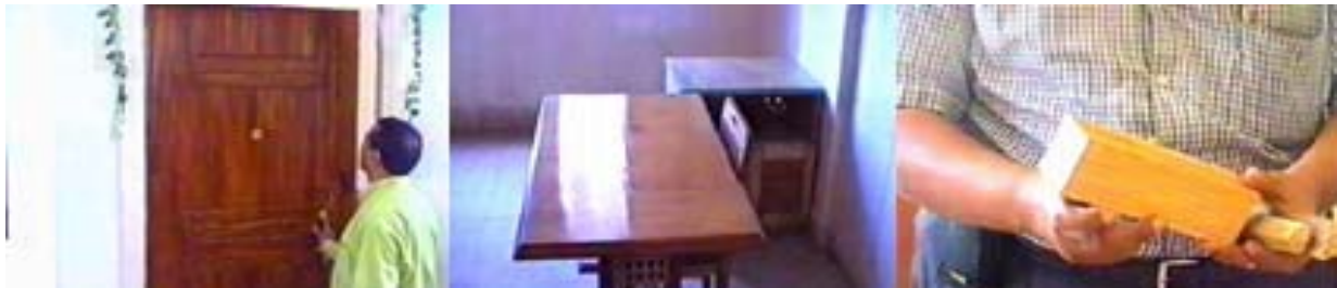
Photo (6.7): Producing blocks of wood from DPLM and some products produced from them
