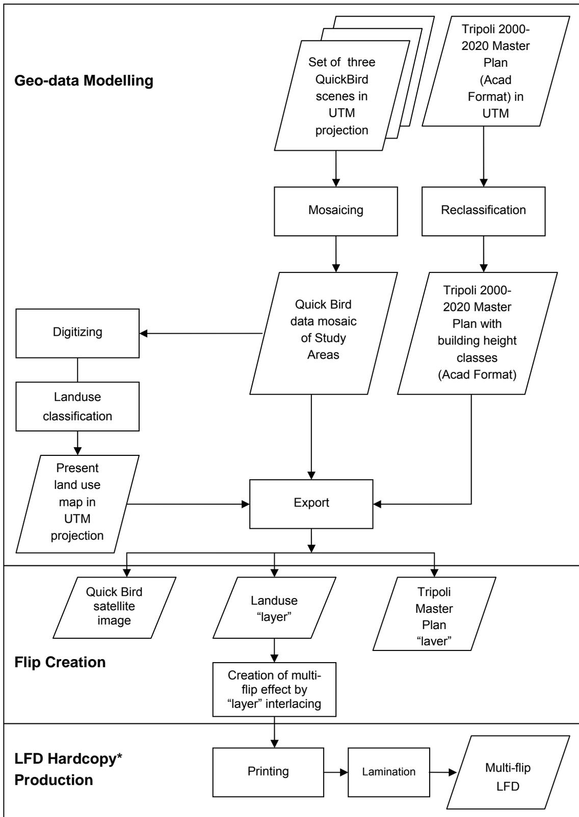
**Figure 5.5: Flow-chart of multi-flip LFD production**
