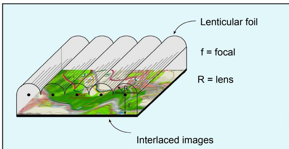
**Figure 5.1: Principle of LFD technology**
