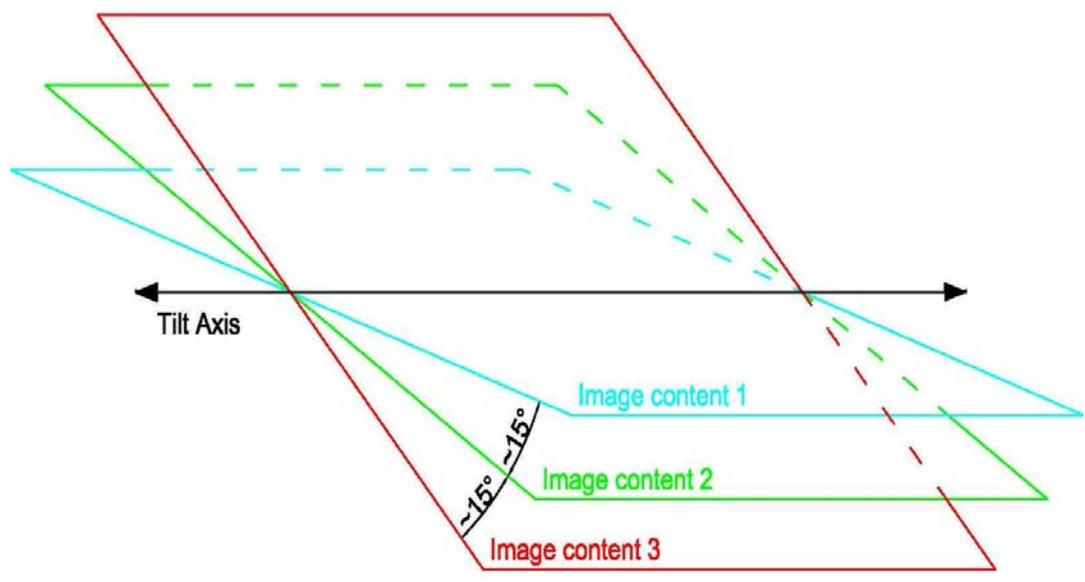
**Figure 5.4: Sketch showing the functioning of a multi-flip LFD with horizontal tilting (cf. Appendix C.1: A, D + E)**
