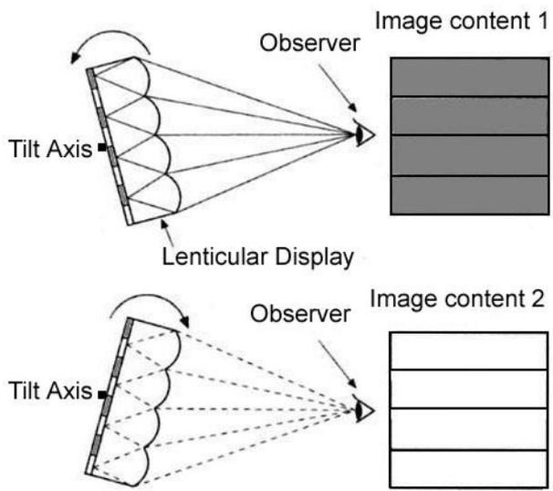
**Figure 5.3: Principle of LFD flip effects**
