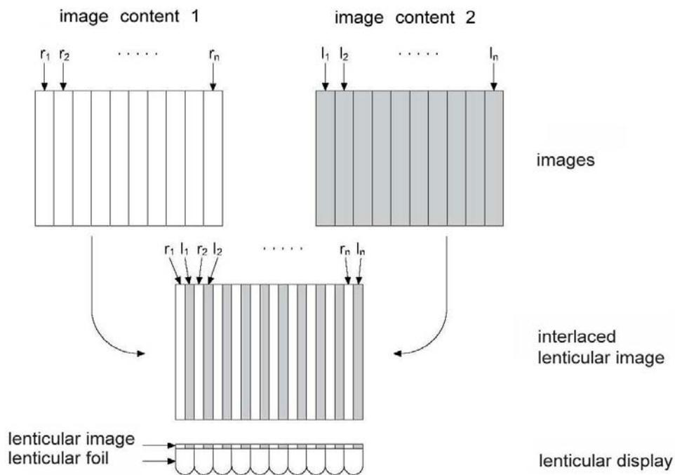
**Figure 5.2: Interlacing of two different images for a 2D flip effect based on LFD**
