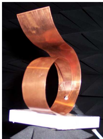
Figure 4.22: A fabricated prototype of the antenna.
