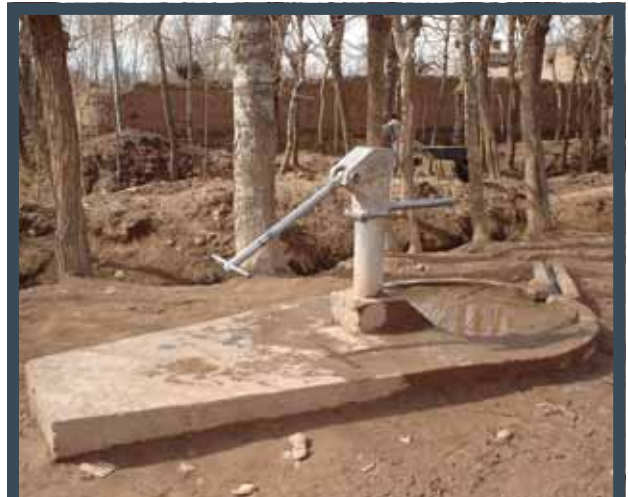
Illustration 16: Well handpump (Bob Rout photograph)
