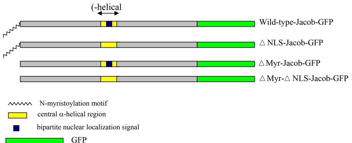
**Fig. 4 Schematic representation of the Jacob cDNA constructs.**
