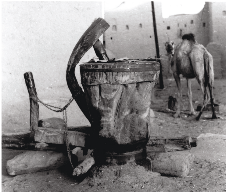
Figure 56. Sesame oil press (see Chapter 3, Section 3.8).
