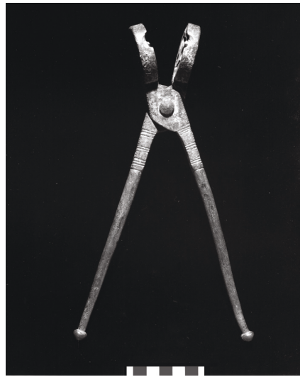
Figure 42. A mould for casting 5 bullets 1.4 sm each. Khuraykhar. The early 20 c. Museum of anthropology and ethnography, St. Petersburg, collection 6920-20.
