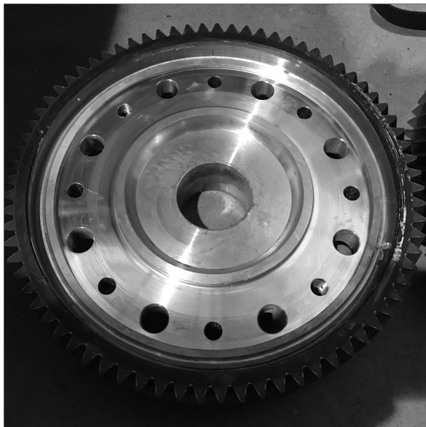
Figure 59: Lightweight gear wheel combining a toothed ring of hardened steel and a softer aluminum alloy core
