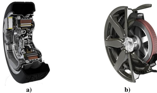
Figure 1: a) Wheel-hub motor from Schaeffler AG [14], b) Demonstrator of Fraunhofer LBF [19]
