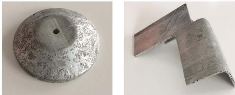
Figure 10: Examples of metal foam structures without cover layers
