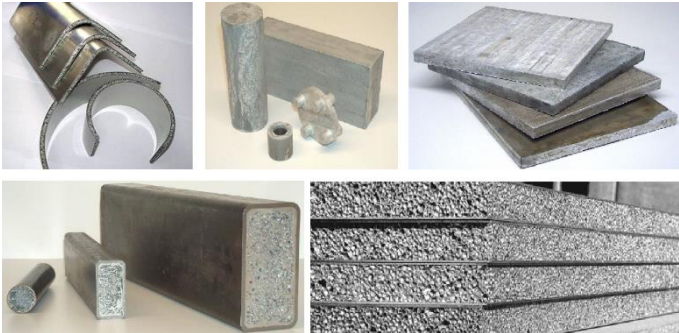
Figure 4: Variety of products based on metal foam sandwich technology
