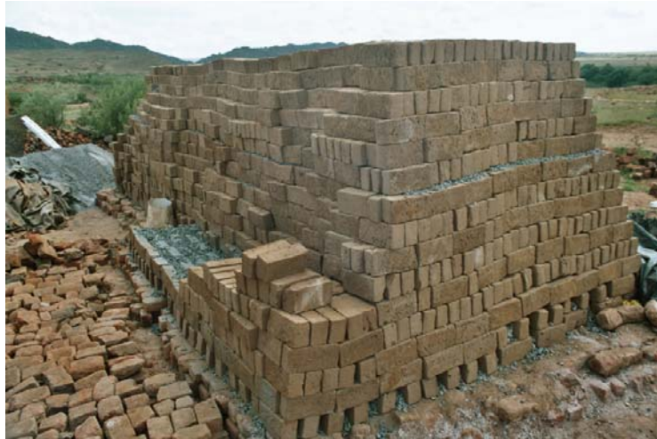
Figure 1.3: Brick stack shortly before completion [4]
