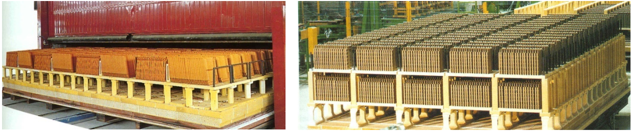
Figure 5.2: Vertical setting for the roof tiles on the kiln car with kiln furniture [3]
