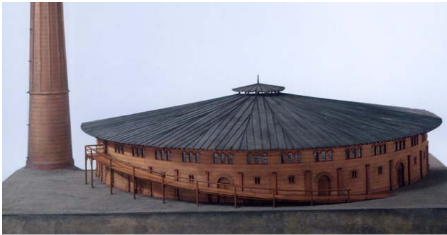
Figure 1.6: Outside appearance of a Hoffmann Kiln [7]
