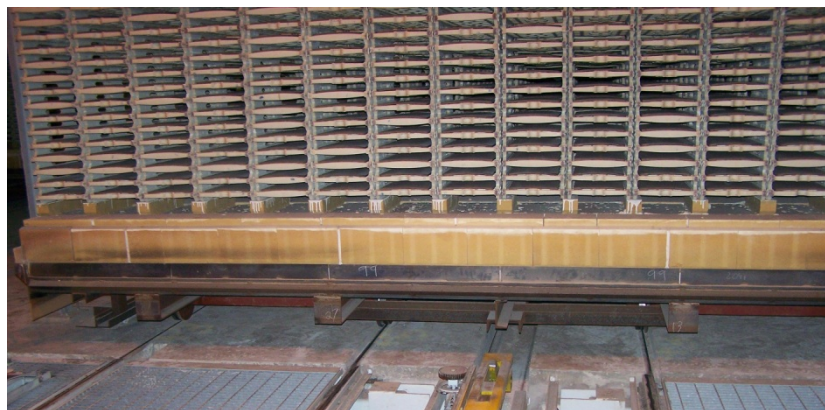
Figure 5.1: Horizontal setting for roof tiles in kiln car with kiln furniture [3]
