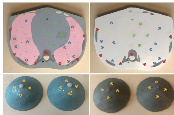
FIGURE 5 Conventionally produced (left) and printed (right) phantom slices and breast add-ons (the printed add-on on the right side contains the glandular structure). For the printed phantom slice, there is no individual color coding for the lung tissue, and the infill pattern is not directly visible because the phantom slice is sealed with a thin layer of fully printed material. The positions for insertion of TLDs are marked with colored circles (red = bones, blue = lungs, green = muscle, yellow = breasts).
