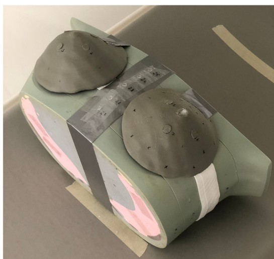
FIGURE 3 Experimental setup for the chest CT scan of the 3D-printed phantom parts (printed slice in the middle). A similar scan containing the conventionally manufactured phantom parts was additionally performed.
