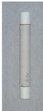
Figure 3-2: Insulated specimen at top and bottom
