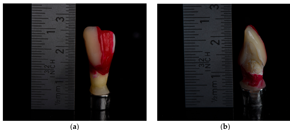
Figure 3. (a,b) Embedded specimen with an already bonded 3D-printed restoration on half of the tooth and prepared with nail varnish covering before placement in demineralizing solution. The approximal areas were not covered with nail varnish in order to expose these areas to the demineralizing solution.
