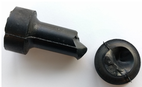
Figure 11.2: A crack propagation due to high stresses at the corner lead to sample failure. Material failed after 705s.
