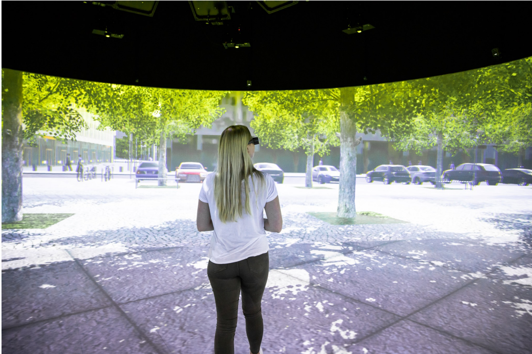
Figure 3.1: Picture from inside the Elbedome. The person wears VR glasses which enables the 3-dimensional viewing of the projection coming from the roof-mounted projectors[3].
