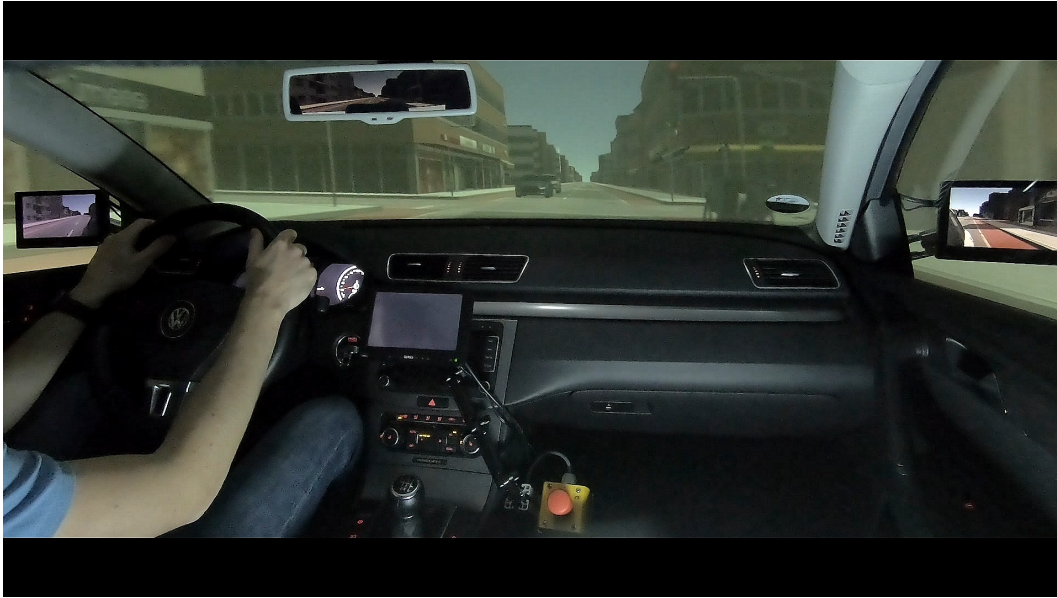
Figure 3.2: Segment from a recording during a scene in the driving simulator. On the right side drives the AuRa bike.
