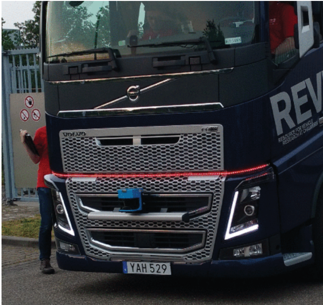
Figure 2.11: Example of an LED strip attaching to the front of a truck from Benderius et al., best-rated human-machine interface that was presented during the 2016 Grand Cooperative Driving Challenge[45]
