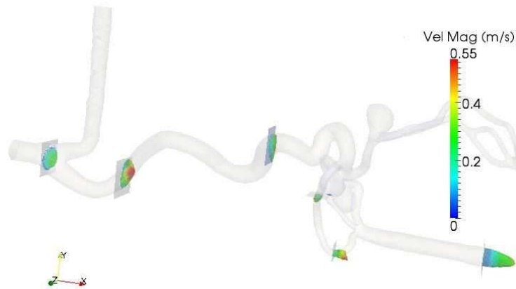
Fig. 3.7.4. Example results from CFD simulations: instantaneous velocity magnitude at different planes within the phantom model at peak pressure
