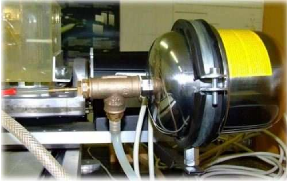
Fig. 3.4.3. The pressure condenser/Windkessel
