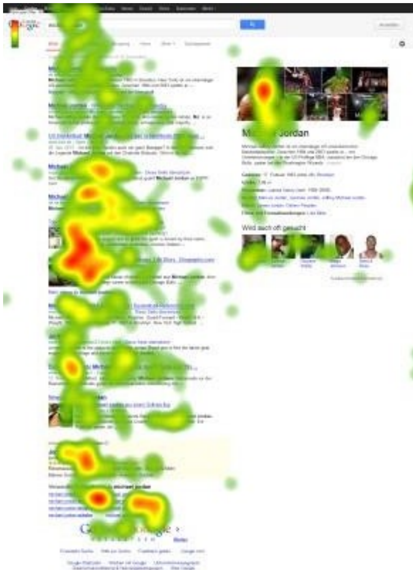
FIGURE 2.6: Taken from [48]: Heat-Map of aggregated fixations to high-light the eye movement on the search engine result page of Google.
