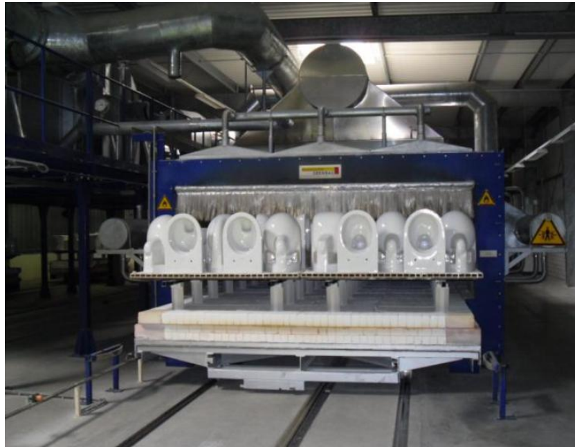
Figure 1.11: Tunnel kiln new conception (this photo had been taken at KERAMAG Company).
