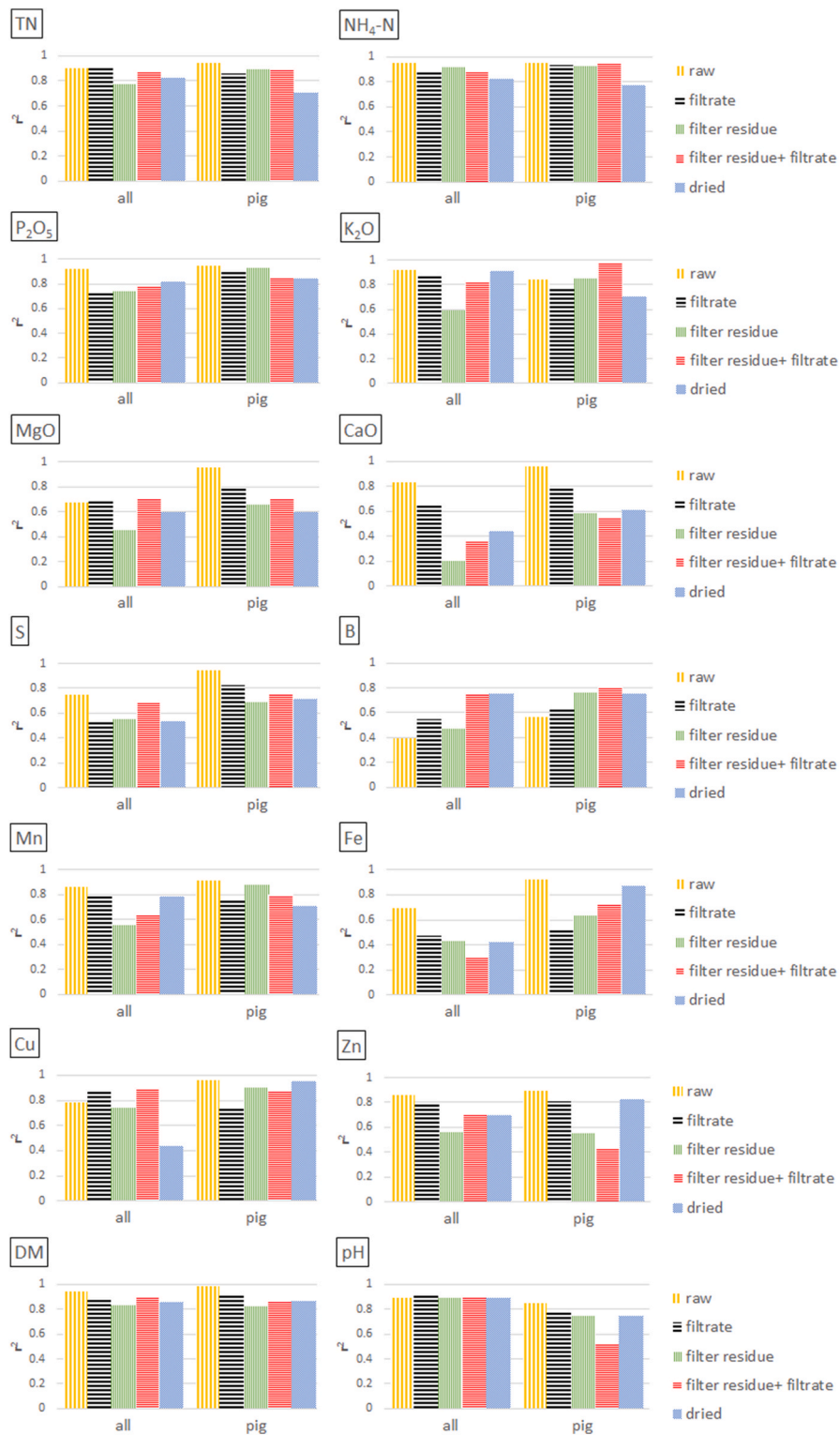
Fig. 3. Calibration model performance ( r^2 ) for LOM properties depending on sample pre-treatment technique (subsamples 1a–1d; see chapter 2.3) and combination of filter residue and filtrate spectra. Concentrations are referring to a wet weight basis. Data set 1 was used, which includes 41 pig, 11 cattle, and 10 digestate LOM samples. Filter residue = wet filter residue representing the solid phase separated by filtration; filter residue + filtrate = combination of spectra from the solid and liquid phase.
