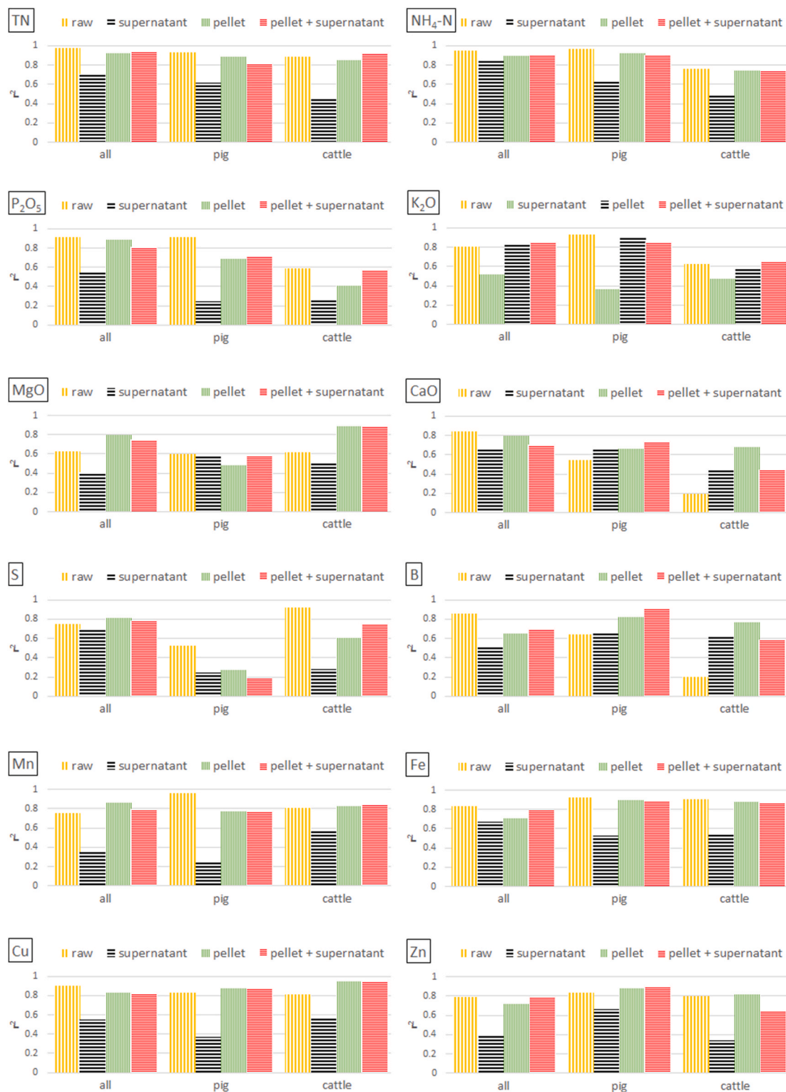
Fig. 6. Calibration model performance ( r^2 ) for LOM properties on dry weight basis depending on sample preparation technique (subsamples 2a–2c; see chapter 2.3) and combination of pellet and supernatant spectra. Data set 2 was used, which includes 50 pig, 51 cattle, and 10 digestate LOM samples. Raw = no treatment; pellet = wet pellet representing the solid phase of LOM separated by centrifugation; supernatant = liquid phase separated by centrifugation; pellet + supernatant = spectral combination of the solid and liquid phase.
