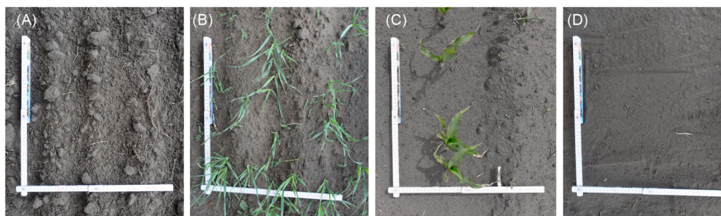
Fig. 5. The initial surface roughnesses: rough cloddy seedbed after steppe conversion on Plot 1 (A), a weak crust on Plot 2 grown with barley (B), and loose material in the rows of maize on Plot 3 (C). The surface roughness without plants and after applying high mechanical stress on Plot 3 (D). The folding ruler is 0.4 \text{ m} \times 0.4 \text{ m} , showing an area of 0.16 \text{ m}^2 .
