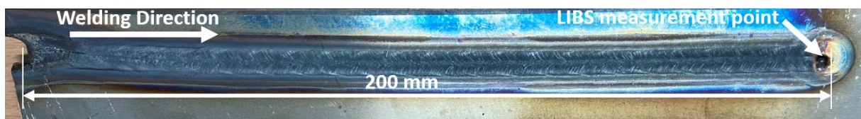
Figure 6-31: Finished weld seam of the Sample 3, LIBS measurement spot on the weld end crater is marked.
