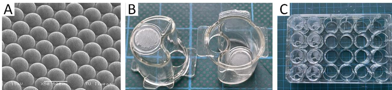
**Fig. 1** 3D cell carrier MatriGrid® and semi-active insert system. **A** Scanning electron microscopy image of apical MatriGrid® direction with porous cavities. **B** MatriGrid®s welded into the semi-active insert systems. **C** 24 well plate filled with semi-active insert systems
