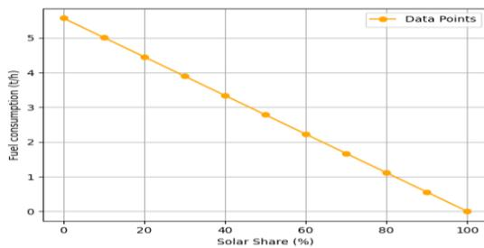
Figure 5: Fuel consumption-Solar share of 28.1 MW SHGT.
