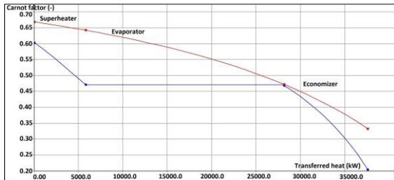
Figure 4: Carnot factor-Energy diagram of HRSG.
