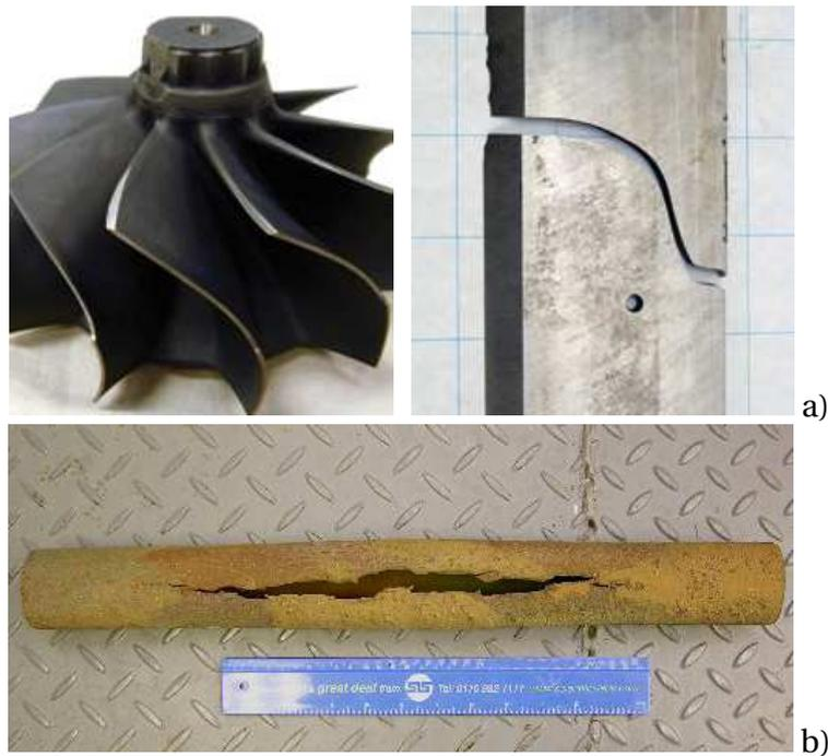
**Figure 1.1** Examples of constructions, fractured due to creep: a) the blade failure due to many processes including creep cavitation (taken from <http://www.atslab.com/>); b) creep fracture of a superheater (taken from <http://www.surescreen.com/scientifics/>)
