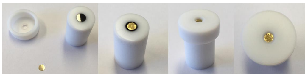
SI Figure 1. Representation of the sample holder for the Au-finder grids with a costume made PTFE cap.
