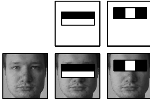
Figure 3.12: The first and second “best” Haar-like features. The first feature represents the difference in intensity between the eyes region and the region across the upper cheeks. The second feature represents the intensity difference between eye regions and the region across the nasal bridge
