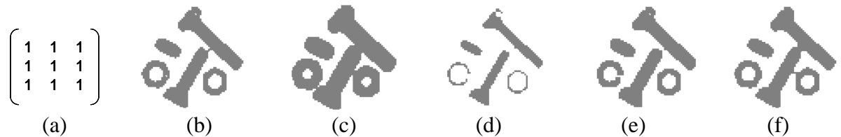
Figure 3.6: (a) Structuring element, (b) original image, (c) after dilation, (d) after erosion, (e) after opening, (f) after closing
