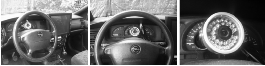
Figure 4.28: NIR camera mounted to the dashboard of the experimental car
