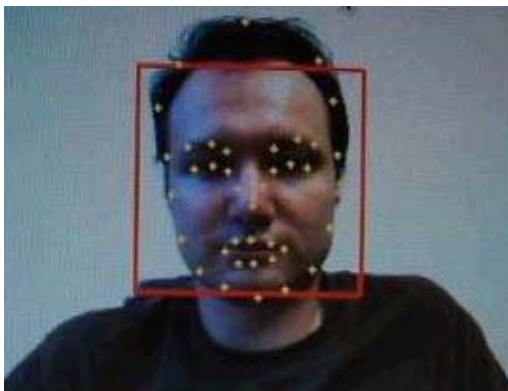
Figure 4.29: Fiducial points and face rectangle localized by Luxand FaceSDK
