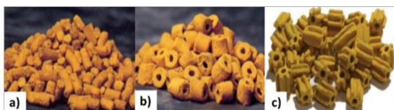
Figure 3: Shapes of the vanadium pentoxide catalyst. a) Pellets, b) Rings, c) Stars [8]
