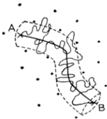
Figure 3.2: Chain segment AB in a dense rubber. Points A and B denote the cross-linked points, and the dots represent other chains which, in this drawing, are assumed to be perpendicular to the paper. Due to entanglements, the chain is confined to the tube-like region denoted by the dashed line. The bold line shows the primitive path. Reproduced from Ref. [141] with permission from the Royal Society of Chemistry.
