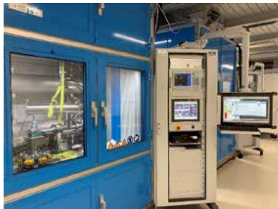
Figure 6: MPI gas valve functional test bench at Bosch Linz
