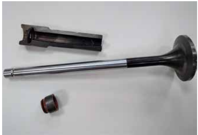
Figure 22: valve, guide with stem cap and seal-ring
