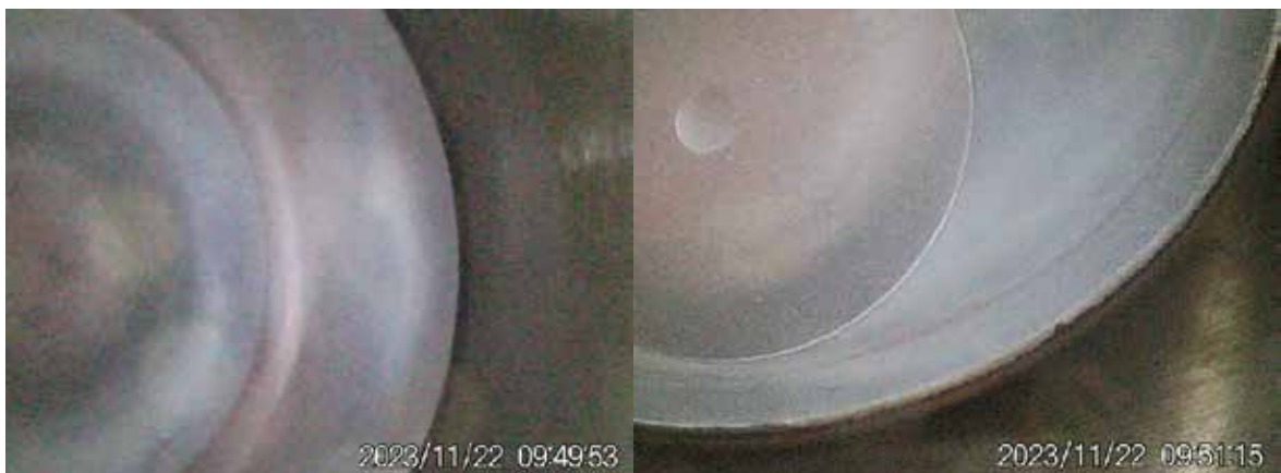
Figure 23: combustion chamber endoscopy of piston and firebox cover
