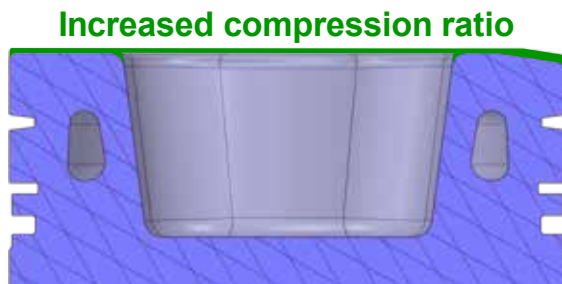
Figure 7: New aluminum piston with increased compression ratio
