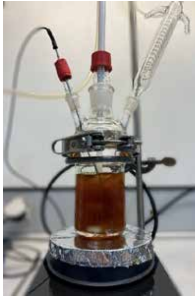
Figure 3: Laboratory scale artificial oil ageing.
