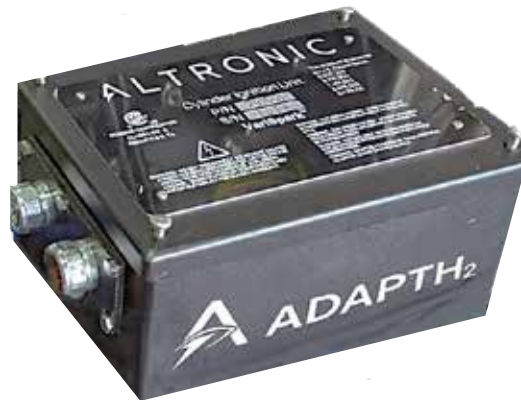
Figure 17. Adapth 2 alpha prototype used for the same-cycle adaptive spark control
