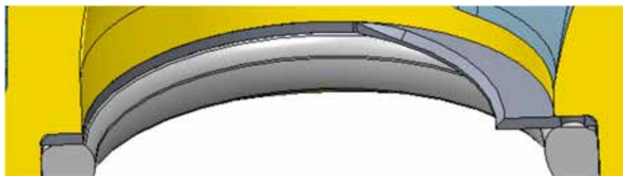
Figure 7: Cut through intake port with tumble blend.
