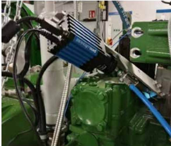
Figure 28: UV camera with combustion chamber endoscope
