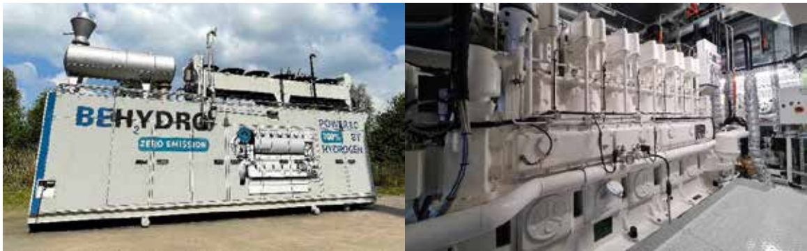
Figure 3. ABC 6DZ hydrogen engine selected for this study and used in marine propulsion
