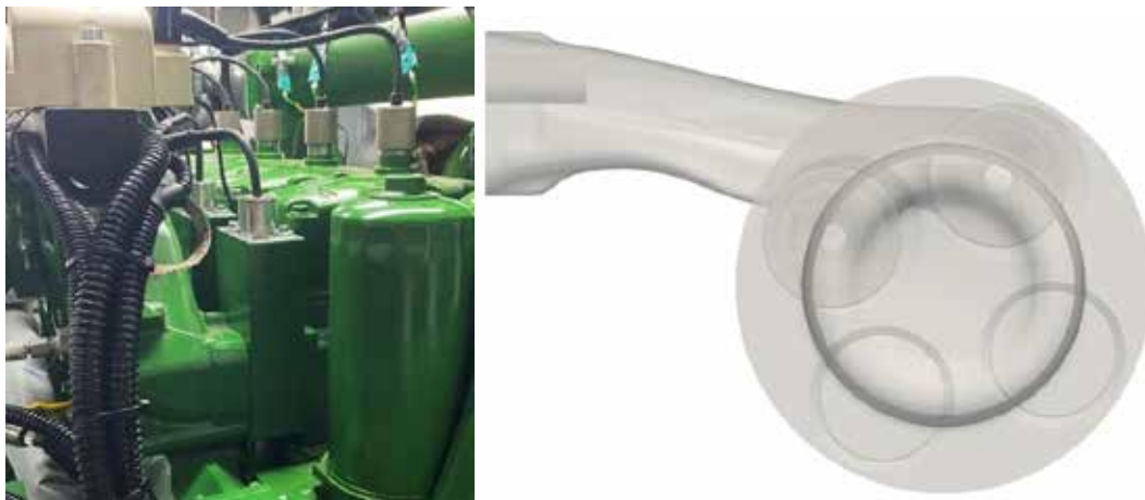
Figure 17: gas intake via hydrogen injector (MPI)
