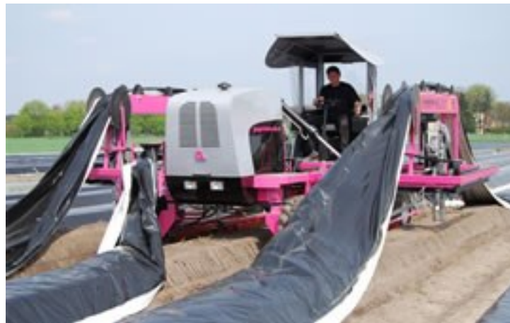
Fig. 1.4: Selective harvesting machine – Panther (from website of top agraronline).
