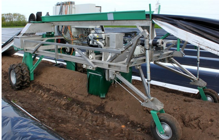
Fig. 1.6: Automatic asparagus harvester 'AutoSpar' (from University of Bremen).
