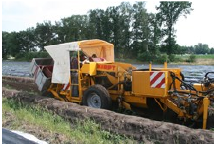
Fig. 1.3: Non-selective harvester Type RGA by Firma Kirpy for white asparagus (from website of ai-solution agrarmaschinen ).
