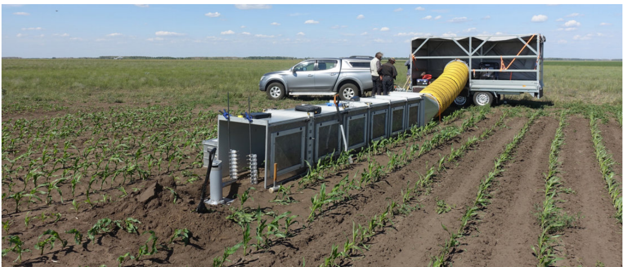
Fig. 4.4. The mobile wind tunnel with MWAC samplers and SUSTRA for collecting aeolian sediments during field experiments on maize.
