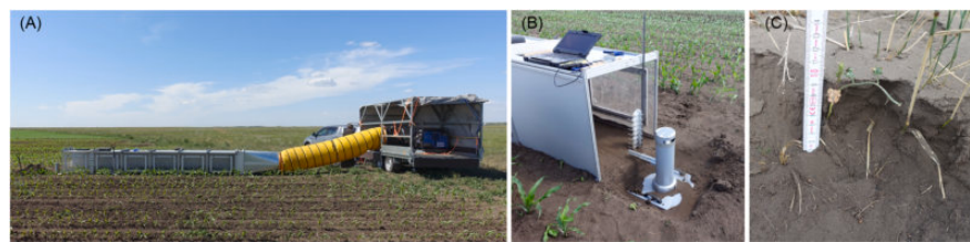
Fig. 4. The mobile wind tunnel during experiments on maize (A), MWACs and SUSTRA for collecting aeolian sediments at the wind tunnel outlet (B), and aeolian depositions from natural wind erosion events on the edge of a field (C).
