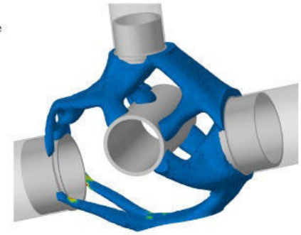
Minimum weight governed by displacement constrain. Colour scale shows life cycles.
