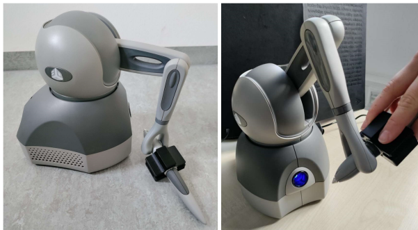
Figure 5.3: Geomagic Touch Device with a 3D printed attachment, mimicking the US probe. Image from Allgaier et al. [9] and available under a CC BY 4.0 license. No changes were made.
