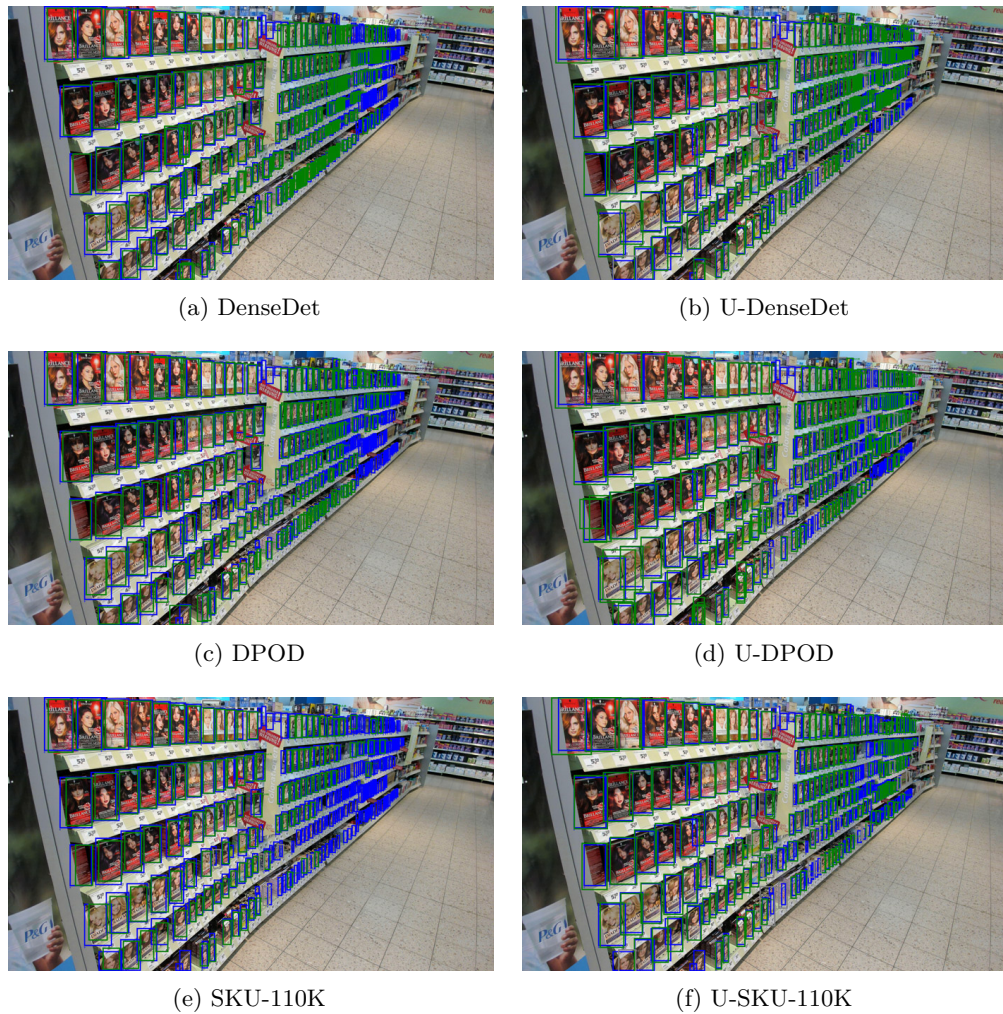
Figure 4.12: Qualitative example of DenseDet, U-DenseDet, DPOD, and U-DPOD on the image frame with id=“bk-03-45”. The left-hand side of the figure depicts state-of-the-art approaches. The right-hand side of the figure depicts the proposed unwarping extension. Correct retail product detections are shown in green. Note how the proposed extension significantly increased the ratio of correctly detected retail products that are more distant from the camera.
