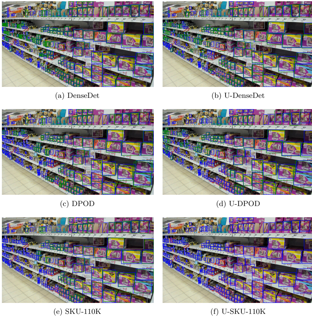
Figure 4.13: Qualitative example of DenseDet, U-DenseDet, DPOD, and U-DPOD on an image frame with id=“sft-10-160”. Images are ordered as before. This is one of the most challenging examples from the MDG-manual dataset. Products significantly varied in scale across the entire shelf. U-DenseDet produced the best results.
