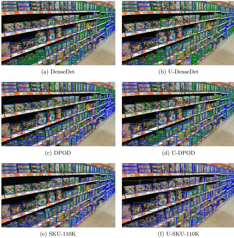
Figure 4.11: Qualitative example of DenseDet, U-DenseDet, DPOD, and U-DPOD on the image frame with id="bk-05-215". The ground truth is depicted as blue bounding boxes. Predictions of each network are shown in gray, but only if the predicted confidence score was greater than 0.5. Correct predictions ( IoU > 0.5 ) are shown in green. Note that U-DenseDet and U-DPOD produced significantly more and better results for relatively small products (right hand side of each image), whereas U-SKU-110K failed to produce good results in this image.
